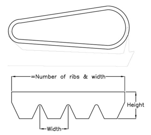
$\begin{array}{ll} \text{Datum Llength} = 1715 \\ \text{Height} &= 9.5 \\ \text{Number of ribs} = 6 \\ \text{Pitch} &= 4.7 \end{array}$
